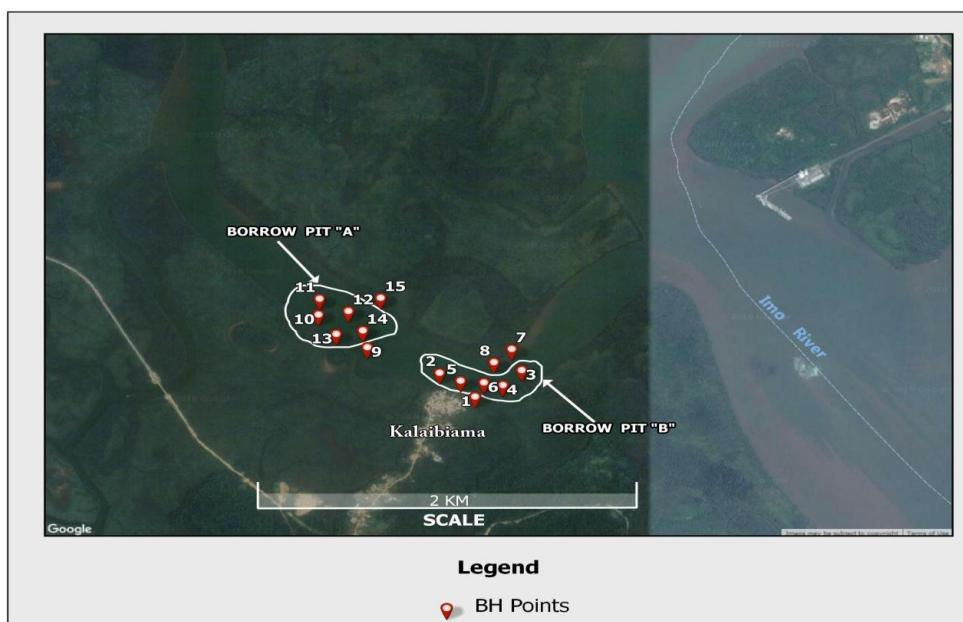
Figure 4: Satellite Imagery showing Location of all Boring Points
