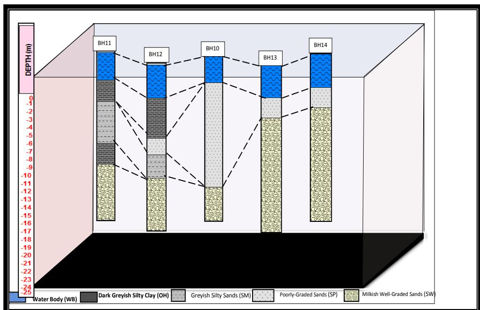
**Figure 3a: Fence Diagram of Strata Logs of Borrow-Pit A**
