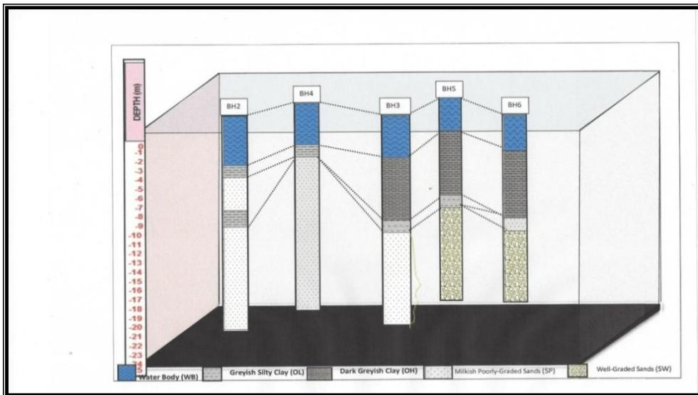
Figure 3b: Fence Diagram of Strata Logs at Borrow-Pit B
