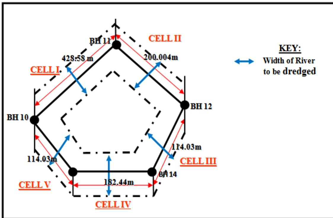
**APPENDIX A 2: Schematic Cross-Section of the Project Site Showing Boring Locations, Actual Distances and Approximate Width of Creeks at Borrow Pit “B”**
